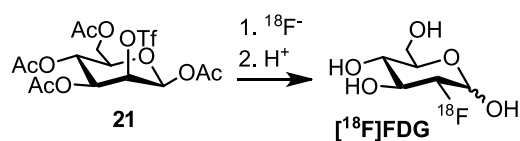
Scheme 4.1 Synthesis of radiotracer [ 18 F]FDG from mannose triflate derivative 21 with nucleophilic 18 F - , developed by Hamacher et al. [216]
