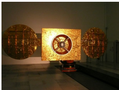
Figure 7.2. Picture of the satellite mockup used for the experiments. The central body of the mockup is 2.3 \times 1.8 m in size. It is wrapped in a MLI-like thermal blanket. The apogee nozzle represents the rear of a typical geostationary satellite.
