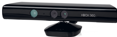
Figure 8.1. The Kinect sensor. An infrared emitter projects a pattern into the scene, which is captured by a camera. Similar to stereo vision, the disparity is used to obtain the distance measurement. ( Image from Wikipedia, public domain )
