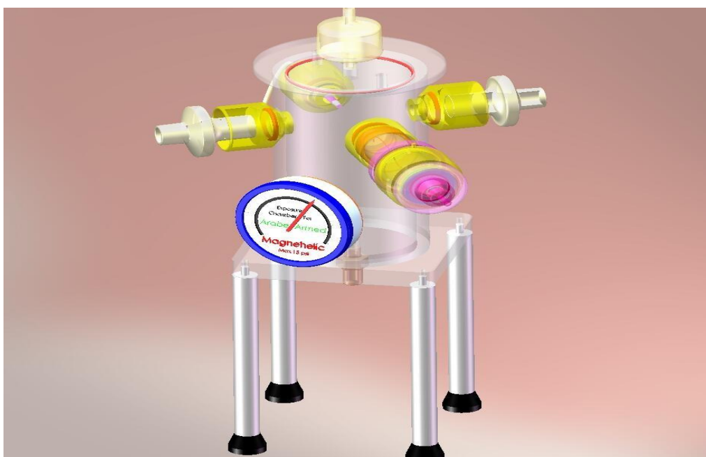
Figure 66: Schematic of the four-port exposure chamber, used for evaluation of the in vitro rat model. Reproduced with permission from Aztec Precision Engineering, Letchworth, UK
