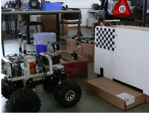
Figure 5.2: Experimental setup for determining the relative transformation between iSpace and camera systems.
