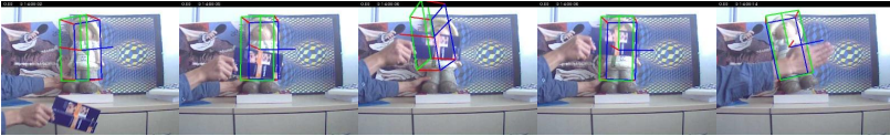
Figure 5.10: The estimated pose under occlusion. The pose estimation is performed with the occlusion objects about 30 cm closer to the cameras than the target.
