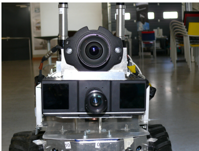
Figure 1.3: Setup of the fused cameras. An AXIS color camera is mechanically mounted on the top of a CamCube2.0. The data from both cameras are fused with the fusion algorithm.
