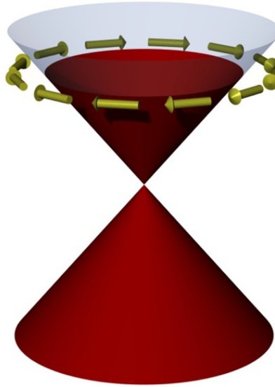
Figure 1.3: Schematic sketch of the single Dirac cone surface state of a 3-dimensional topological insulator. [30]
