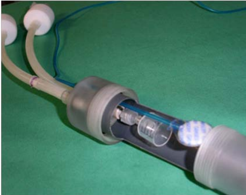
Fig. 3.1: Animal imaging container for magnetic resonance imaging of mice with S. aureus thigh infection. The container was constructed to comply with biosafety level 2 restrictions. Mice were placed on the inner bed and received inhalation anesthesia during the imaging experiment. Heart beat and breathing was controlled with the balloon, which was placed on the chest of the mice.
