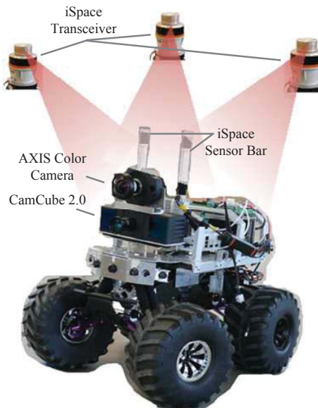
Figure 3.19: Hardware setup on Outdoor MERLIN for formation tracking using visual data, and high-precision measuring unit for evaluation.
