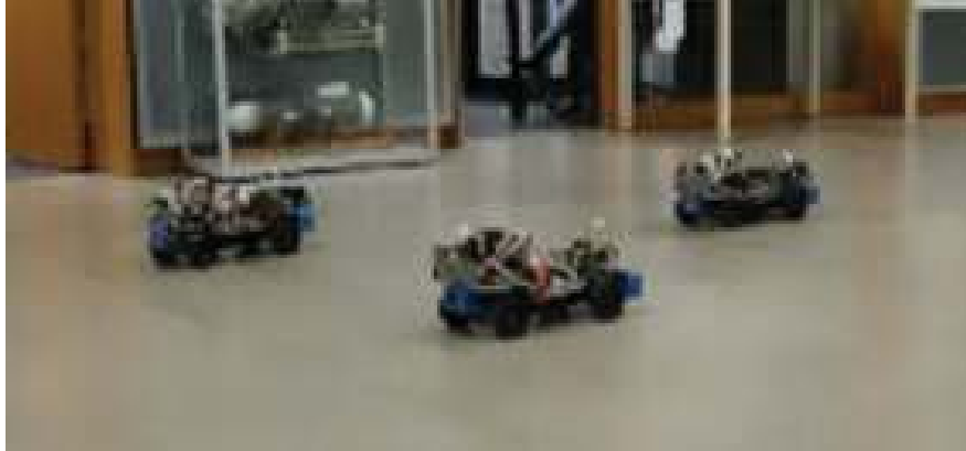
(a) Three MERLIN robots starting the experiment in a V-Formation; the leader robot in front is given the commands to drive straight at this moment.
