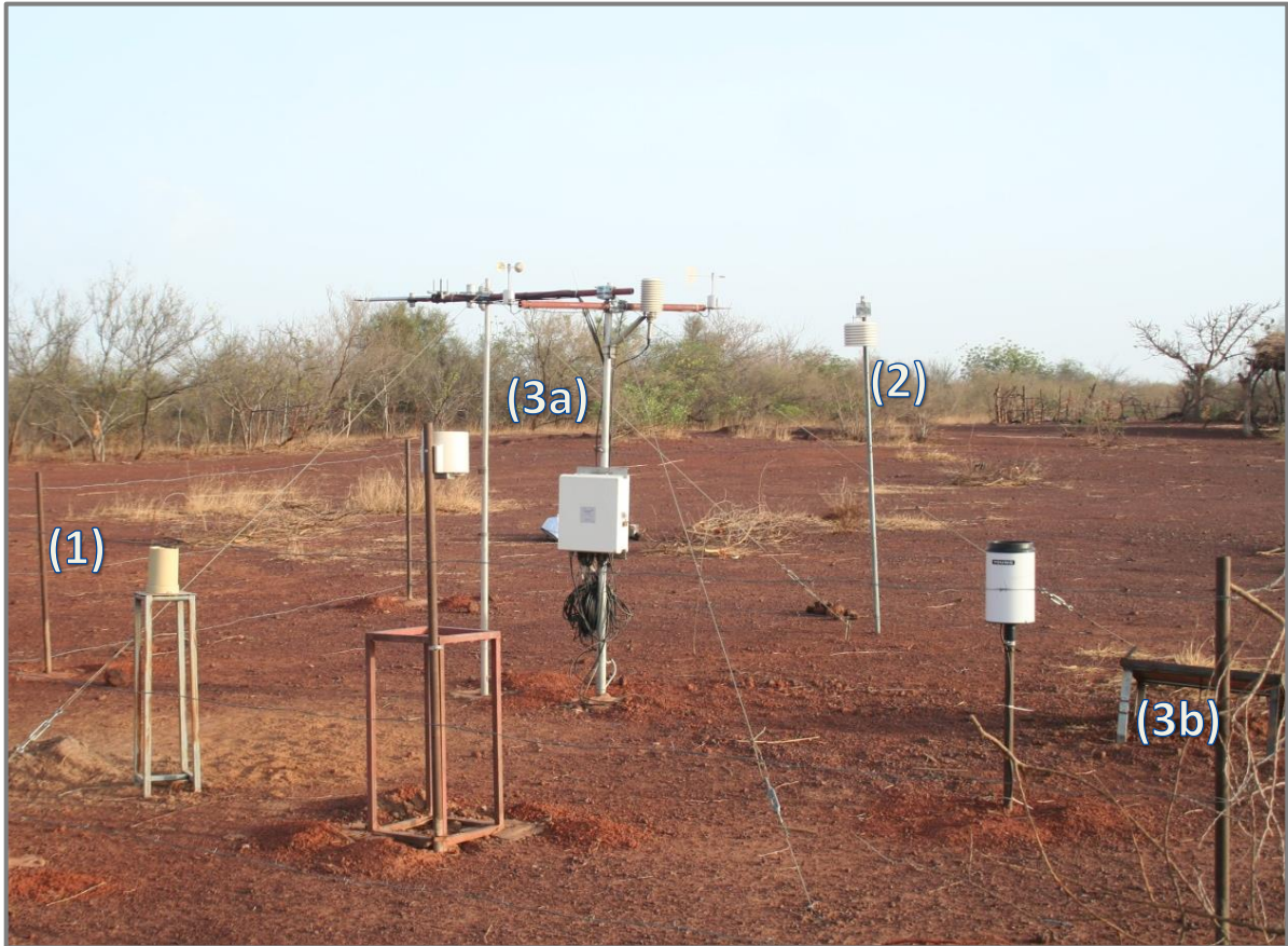
Fig. A4-2: In 2005, a small tipping-bucket rain gauge (1) and a temperature sensor (2) were installed in the degraded site of the Zaï system (sub-Sahel region, Burkina Faso). In 2007, a climatic station (3a) with solar panel (3b) was installed by the climatology group of BIOTA West Africa.
