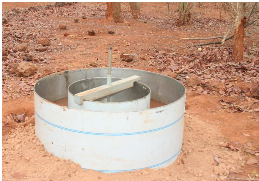
Fig. A8-4: A) Double-ring infiltration conducted simultaneously in a sub-quadrat with recent termite activity (here: compost) and in the control-plot of the same experimental block (degraded area, ZDeg); and B) one of two sub-quadrats in which an infiltration measurement was simultaneously conducted in the young Zaï forest (ZF20) (both dry season 2006). In both photos, Macrotermes mound-soil was used to seal the base of the outer ring. In most cases, the clayey mound-soil had to be used at some point of the measurement to ensure that the water in the outer ring did not start to leak sideward at the rings' base.
