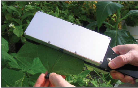
Figure 2-1: Usage of the LI-COR LI-3000 leaf area meter (Adapted from LI-COR, 2006).
