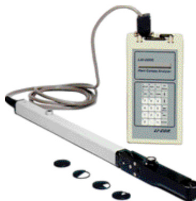
Figure 2-4: The LI-COR LAI-2000 Plant Canopy Analyzer (Source: LICOR, 2005)
