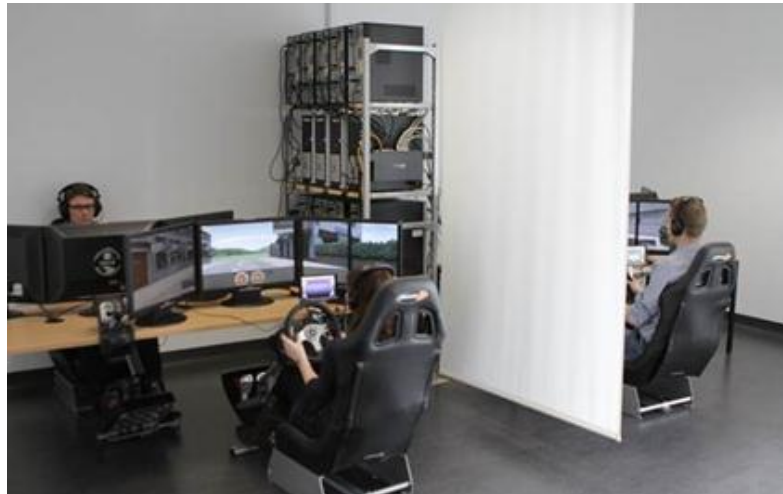
Figure 31. The multi driver simulator. Three of the four driving stations are visible in the picture.
