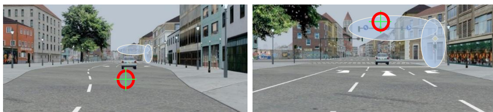
Figure 13. Ellipses around the traffic light defined the traffic light as areas of interest, depicted for two different distances during the traffic light approach. The red circle represents the fixation point as determined by the eye tracker.
