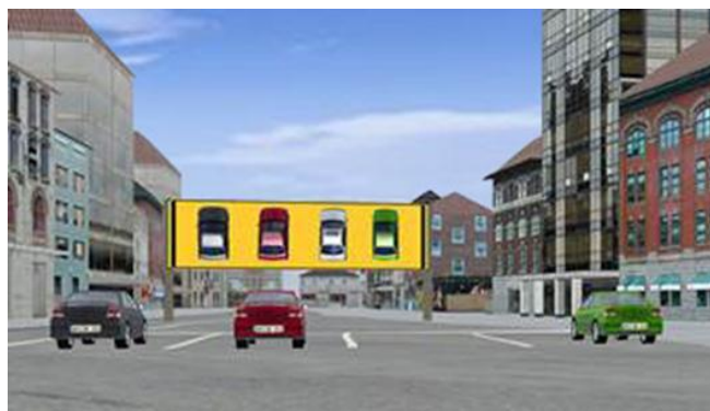
Figure 34. Traffic sign showing the position of the vehicles in the platoon. Drivers parked in the required position and subsequently started the next section of the test track from left to right (also see Mühlbacher, 2013).
