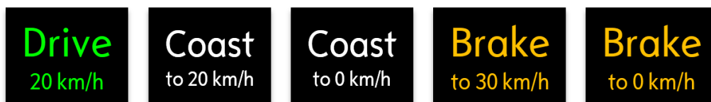
Figure 32. Driving recommendations in the HMI display. “Drive” was depicted in green, “coast” was depicted in white, and “brake” was depicted in amber. The original recommendations contained German text (“Fahren”, “Ausrollen”, and “Bremsen”).
