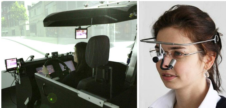
Figure 9. Driving simulator mockup (left, picture from WIVW GmbH) and head mounted eye tracker (right, picture from Ergoneers GmbH).
