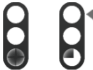
Figure 54. Schema of the traffic light phase information as depicted in the HMI concept. The left traffic light showed the current traffic light state. The right traffic light showed the remaining time in the current traffic light with one quarter representing 2 s. The arrow next to the traffic light highlighted the traffic light phase at which the driver arrived at the intersection (right picture: arrival at red, remaining time in green 2 s).
