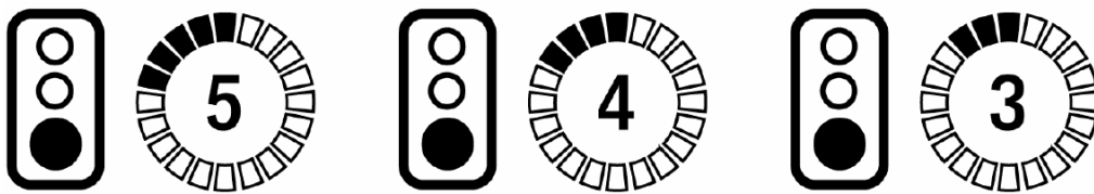
Figure 45. Information about the duration of the current traffic light phase (Thoma et al., 2007).
