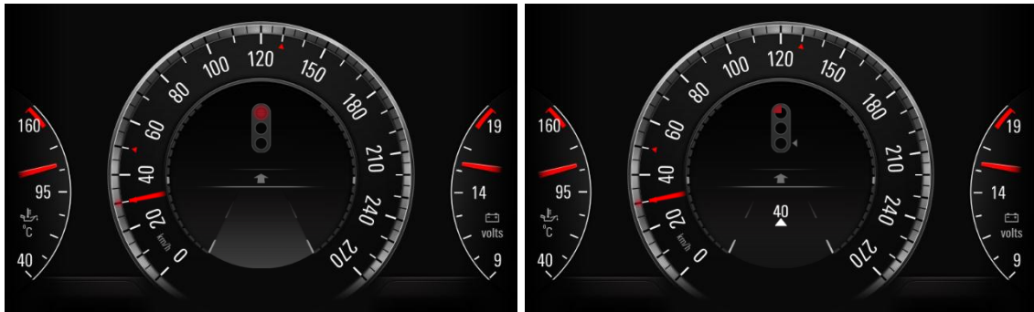
Figure 80. HMI versions as used in the experiment. The simple version showed the current traffic light phase (left). The complex version showed information on the traffic light phase duration, phase at arrival, action and speed recommendations (right).
