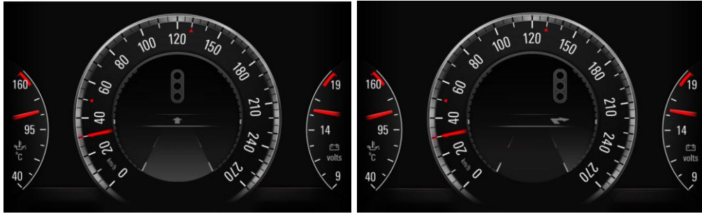
Figure 53. Cluster display with speedometer and basic HMI structure. Information for all three possible driving directions was depicted lane specific by highlighting the lane (left pictures shows driving straight, right picture shows turning right).
