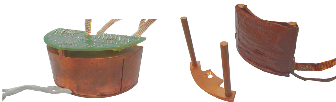
Figure 16: copper powder filters in version 1 (left) with R-C-filtering and version 2 (right)
