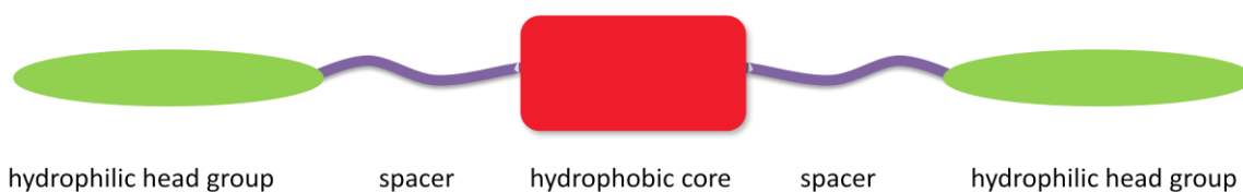
Figure 2. Schematic illustration of a bola-amphiphilic building block: hydrophilic head groups (polar or charged residues) connected via spacers to the central hydrophobic core.
