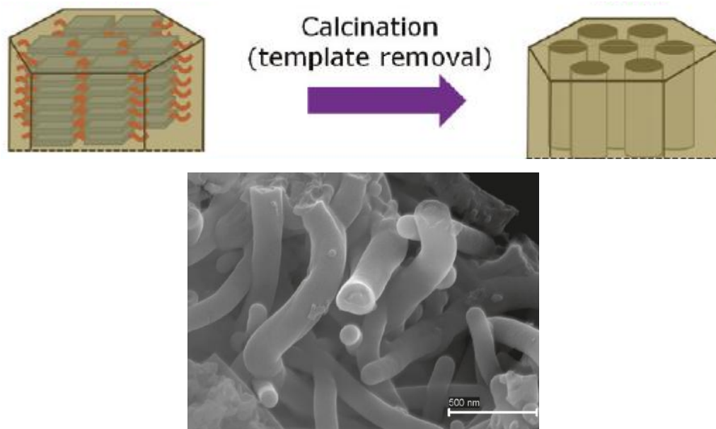
Figure 26. Schematic illustration of the preparation of nanoporous silica (top right) by calcination of a silica-dye nanocomposite (top left). SEM image of calcinated silica synthesized from PBI solution (bottom). Reproduced with permission from ref [69]. Copyright 2011, American Chemical Society.
