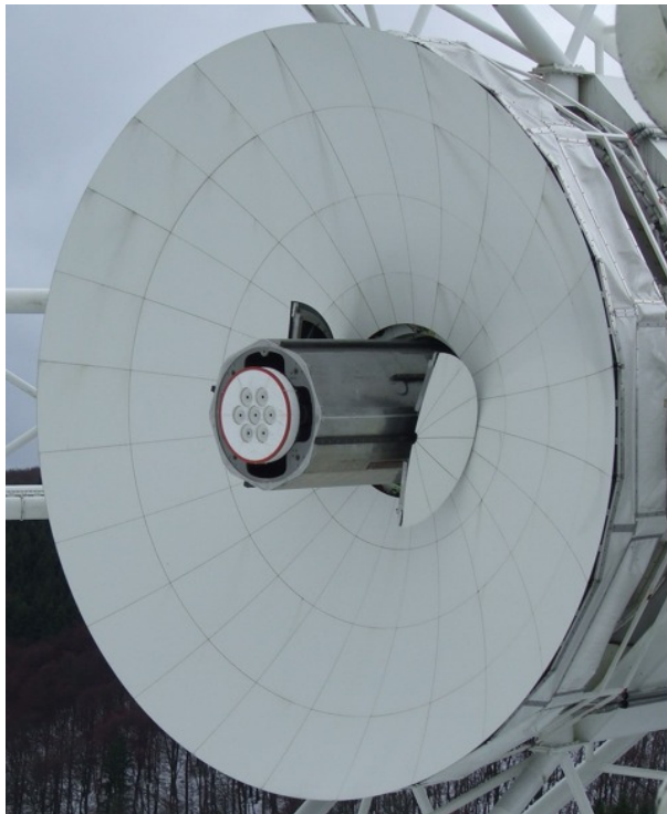
Figure 4.6.: The Seven Beam receiver mounted in the primary focus of the Effelsberg radio telescope (Image Credit: A. Kraus).
