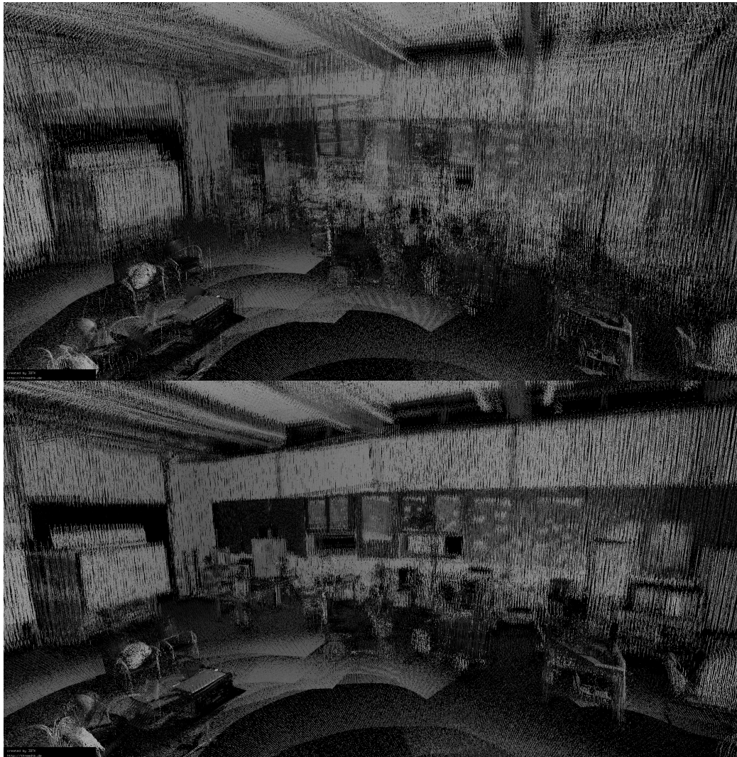
Figure 8. 3D point cloud of Experiment 1 with reflectance values. The quality improves, but the contours are still not sharp after optimization.
