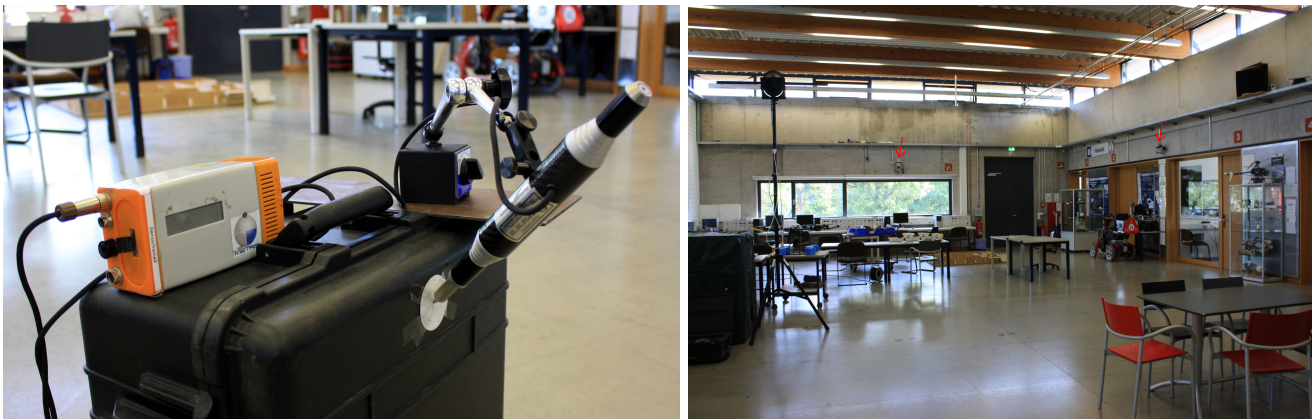
Figure 3. (Left): The positions of the reflective markers in the iSpace coordinate system are measured with the hand vector bar. (Right): the iSpace transmitters are mounted on the walls of the robotics hall at the University of Würzburg, where the experiments were carried out.
