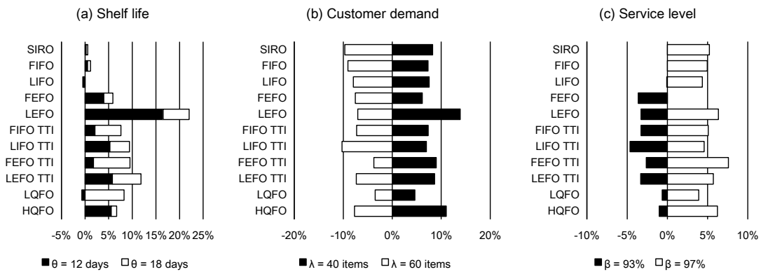
Figure 25. Impact of parameter variations on holding costs for expiry-based customer withdrawal behavior
