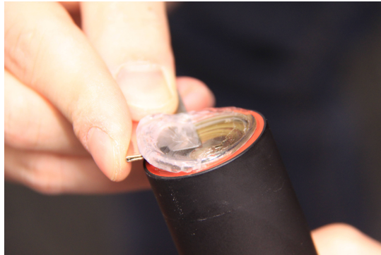
Figure 10.5.: Picture (by Dominik Köth) of removing adhesive remains from a photomultiplier using a razor blade.
