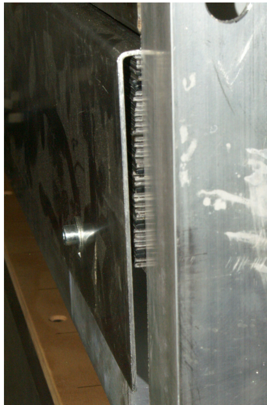
Figure 9.3.: Picture of the absorber showing the internal structure. The 42 steel sheets of the absorber can be seen as well as one of the cover panels, attached for safety reasons.
