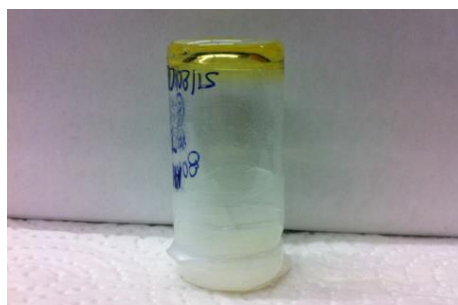
Fig. 85 Photograph showing the “stable-to-inversion of the test tube” method of the hydrogel of 3 in water.
