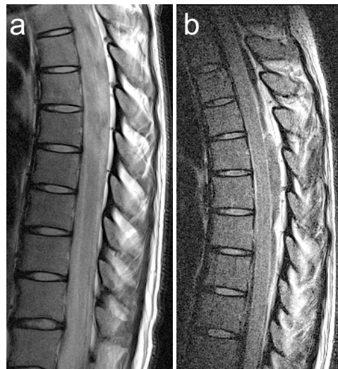
Figure 4.11: In-vivo comparison: conventional mode using the transmit body coil and local spine receive coil (a), high-bandwidth mode applied by the transmit/receive spine coil (b).
