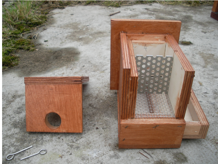
FIGURE 2.2: Pollen trap with removable 5mm hole grid, lid and drawer for collecting the pollen sample. Developed for observation hives of honey bee colonies.
