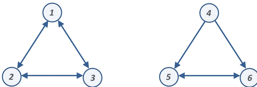
FIGURE 5.4: Communication topology for cluster 1 and 2. Figure adapted from Ref. [5]. © (2016) IEEE.
