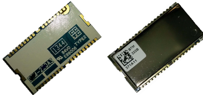
FIGURE 2.2: Bluetooth module BTM-222.
