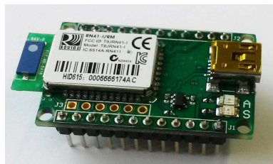
FIGURE 2.3: RN41-I/RM Bluetooth module.
