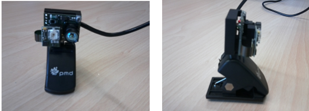
FIGURE 1.8: Front and side view of a PMD camera. Figure adapted from Ref. [1].
