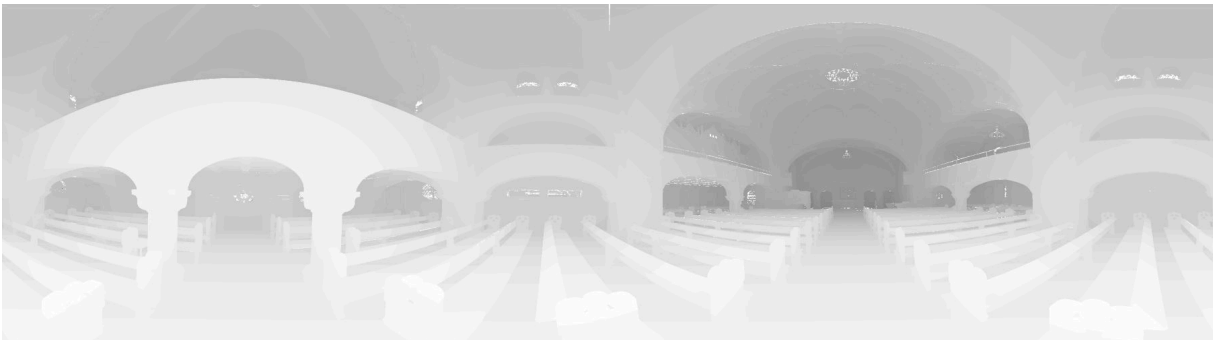
Figure 2.15: Range map of a 3D point cloud. Generated by mapping the 3D point cloud with the Mercator projection onto a panorama image.
