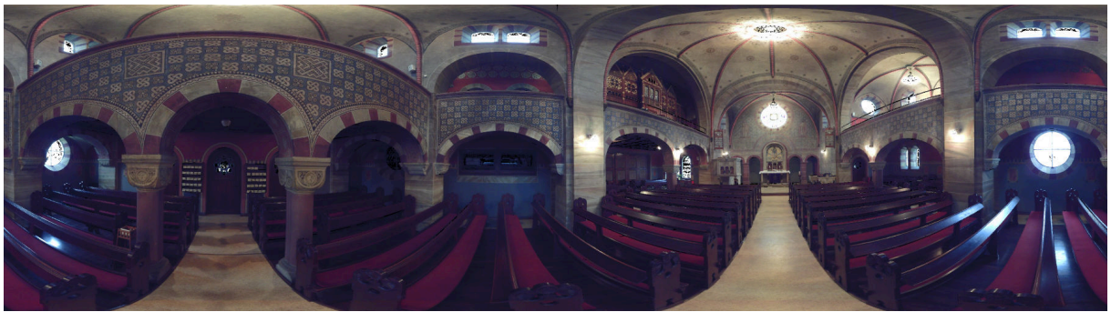
Figure 2.39: Color map of a 3D point cloud. Generated by mapping the 3D point cloud with the equal-area cylindrical projection onto a panorama image. Standard lines at \varphi = -30^\circ and \varphi = 30^\circ are used for generation of this map.
