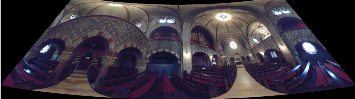
Figure 2.35: Color map of a 3D point cloud. Generated by mapping the 3D point cloud with the Albers equal-area conic projection onto a panorama image. Standard lines at \varphi_1 = -40^\circ and \varphi_2 = 60^\circ are used for generation of this map.
