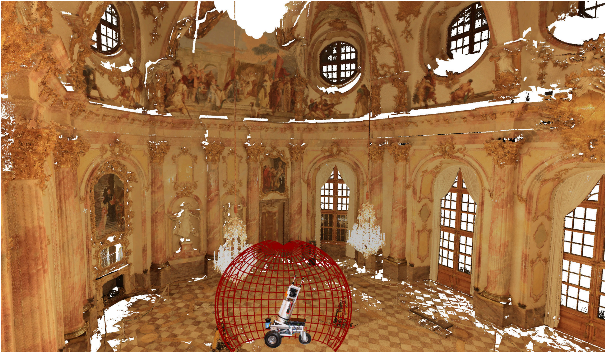
Figure 6.3: Illustration of a 3D scan reconstruction of the Imperial Hall of the Würzburg Residence, Würzburg, Germany. Data is captured by the mobile robot platform (Irma3D) with a VZ-400 laser scanner by RIEGL Measurement GmbH. Attached to the top of the scanner is a Canon 1000D DSLR camera. After a 3D scan has been acquired the camera is used to acquire color information for the point cloud.
