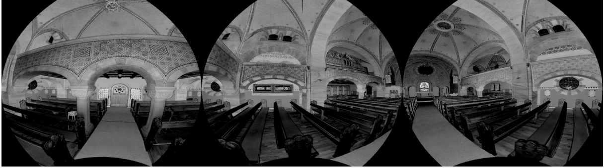
Figure 2.28: Reflectance map of a 3D point cloud. Generated by mapping the 3D point cloud with stereographic projection onto a panorama image.
