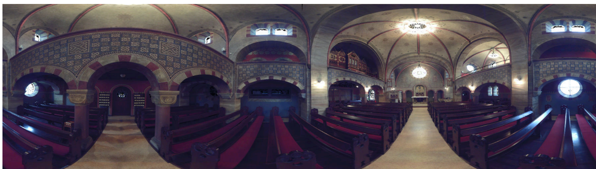
Figure 2.4: Color map of a 3D point cloud. Generated by mapping the 3D point cloud with equirectangular projection onto a panorama image.
