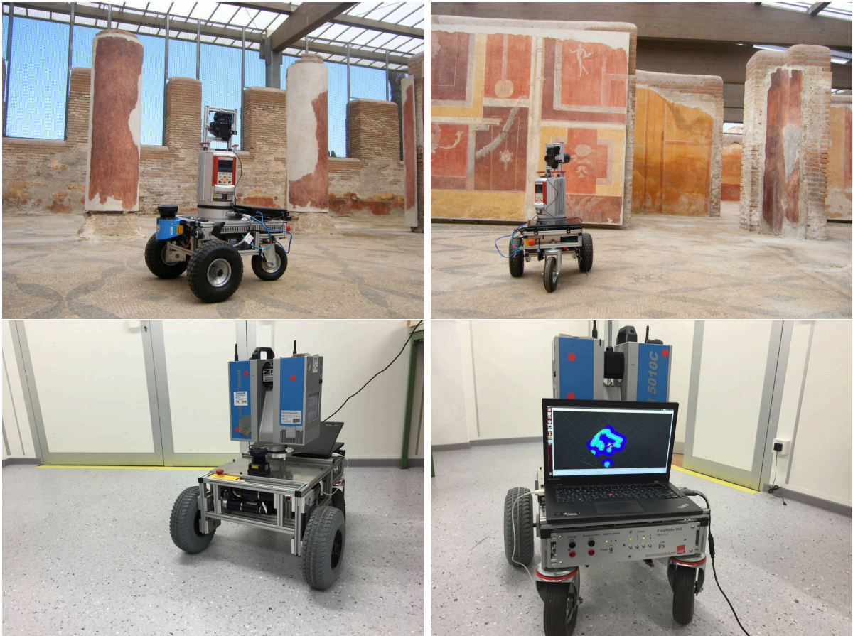
Figure 7.1: These robots are equipped with a differential drive system. Two motorised wheels in the front and one or two castor wheels in the back for stability. Both robots are equipped with 2D/3D laser scanners. Top: Irma3D the three wheeled mobile robot. An additional camera is mounted on the scanner to provide color information for the measured points. Bottom: ZF-Volksbot the four wheeled mobile robot. This configuration allows for higher payloads than the three wheeled configuration.
