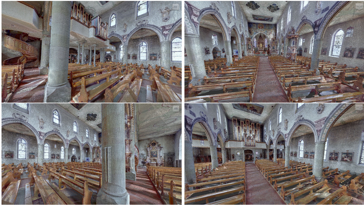
Figure 7.20: Color representation of the registered point clouds from the Saint Martin church in Wangen im Allgäu, Germany. The data set contains 21 scans captured from the inside of the church. The data is captured with Z+F IMAGER 5010C scanner. Each scan contains around 45 million points. The color information is captured with the help of the HDR camera of the scanner. The data is registered and a complete 3D model of the environment is generated.
