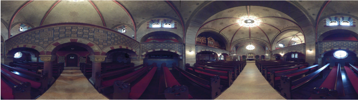
Figure 4.4: Illustration of a colored panorama image generated with the Mercator projection from a sample 3D scan captured from a church in Bremen-Grohn, Germany. The data was captured with a FARO Focus3D laser scanner. The scanner has a built-in camera that captures the color of the point cloud.
