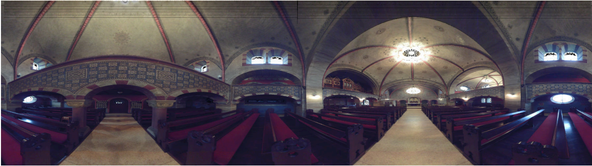
Figure 2.9: Color map of a 3D point cloud. Generated by mapping the 3D point cloud with cylindrical projection onto a panorama image.
