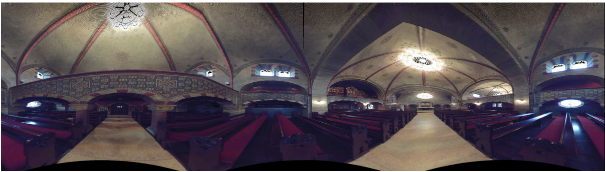
Figure 2.23: Color map of a 3D point cloud. Generated by mapping the 3D point cloud with the Pannini projection onto a panorama image.
