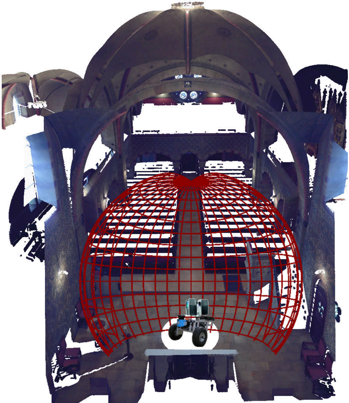
Figure 4.1: Illustration of a 3D scan acquired by a FARO Focus3D laser scanner. The scanner gauges up to 976000 points/sec on a sphere around it by a rotating mirror and a second rotation around the vertical axis. The scanner has a built-in camera and is capable of acquiring color images. Hence, the colored point cloud.
