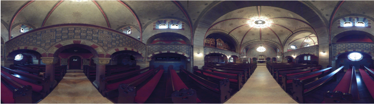
Figure 2.13: Color map of a 3D point cloud. Generated by mapping the 3D point cloud with the Mercator projection onto a panorama image.
