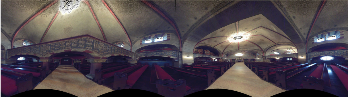
Figure 2.18: Color map of a 3D point cloud. Generated by mapping the 3D point cloud with rectilinear projection onto a panorama image.
