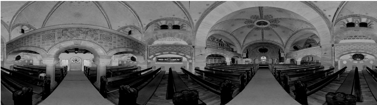
Figure 2.14: Reflectance map of a 3D point cloud. Generated by mapping the 3D point cloud with the Mercator projection onto a panorama image.
