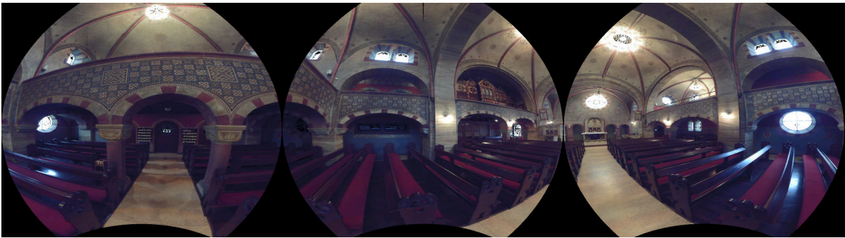
Figure 2.27: Color map of a 3D point cloud. Generated by mapping the 3D point cloud with stereographic projection onto a panorama image.
