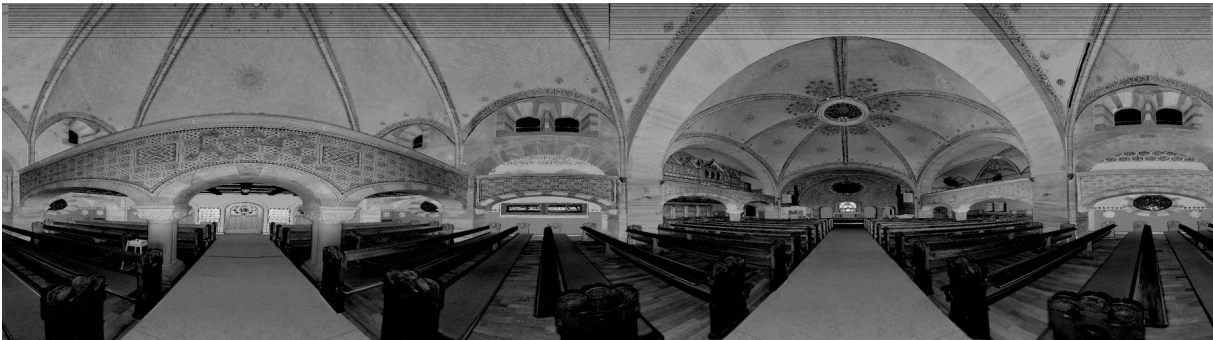
Figure 2.10: Reflectance map of a 3D point cloud. Generated by mapping the 3D point cloud with cylindrical projection onto a panorama image.
