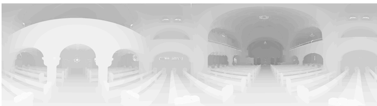
Figure 2.6: Range map of a 3D point cloud. Generated by mapping the 3D point cloud with equirectangular projection onto a panorama image.
