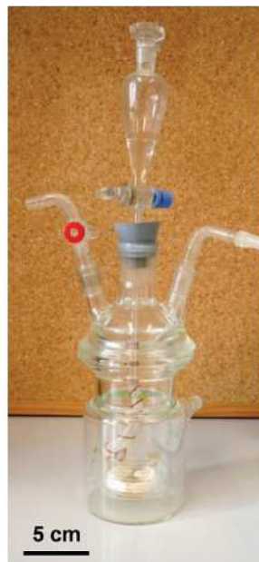
Figure 4.17: Vacuum apparatus for optimal cross linking results containing a meniscus scaffold.
