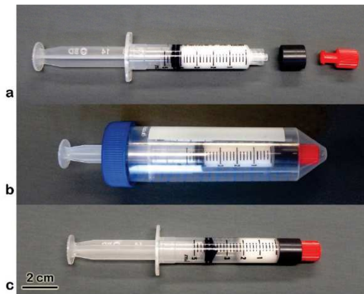
Figure 4.11: Centrifugation of precursors in syringe setup. a) A Luer-Lock syringe filled with precursor (white) is augmented with a stabilization unit (black) and cap-locked (red). b) The system is transferred in a centrifugation tube. c) After centrifugation, a highly effective degassing is achieved.
