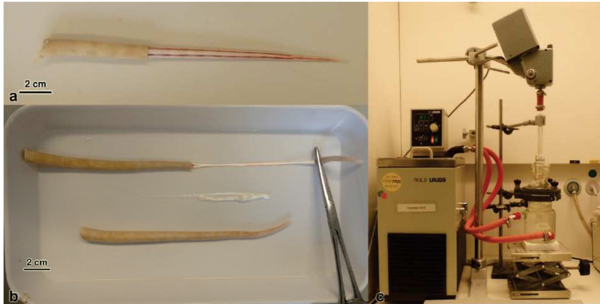
Figure 3.1: Isolation of collagen I from murine tendon. a) Radial orientation of the tendons along a rat tail. b) Pulling out of collagenous tendon material. c) Setup for acidic fractionation of collagen I.
