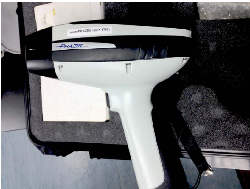
Figure 1: A handheld Raman Spectrometer (photo taken at the Muhimbili University of Health and Allied Sciences). 2
