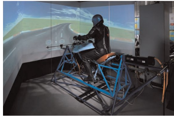
Figure 4: Motorcycle riding simulators for research and development (II). Left: IFSTTAR, France (Nebaoua, Hima, Arioui, Ségué, & Éspié, 2007, p. 180). Right: University of Padova, Italy (Cossalter, Lot, Massaro, & Sartori, 2011, p. 709).
