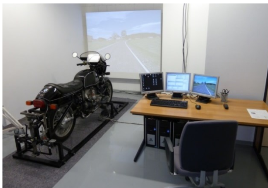
Figure 5: Motorcycle riding simulators for research and development (III). WIVW Static I (left, private picture) and Static II (Will, in press), Germany.
