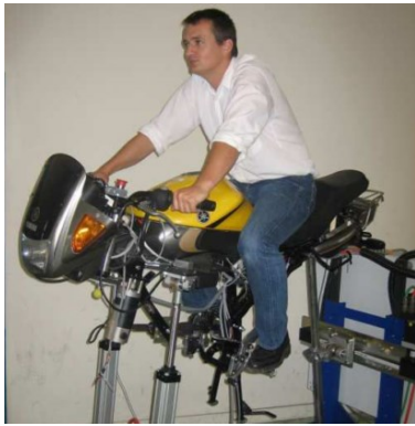
Figure 4: Motorcycle riding simulators for research and development (II). Left: IFSTTAR, France (Nebaoua, Hima, Arioui, Ségué, & Éspié, 2007, p. 180). Right: University of Padova, Italy (Cossalter, Lot, Massaro, & Sartori, 2011, p. 709).
