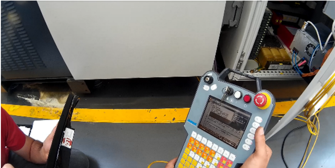
Figure 6.50: Service technician view (head-mounted camera) on teach pendant
