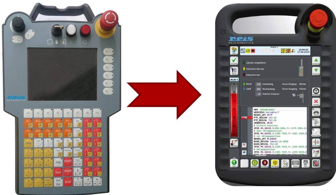
Figure 4.2: Teach pendant (left) of a a Reis/KUKA Industries manipulator and a new reisPAD (right)
