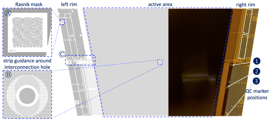
Figure 7.2.: Drawing of a Micromegas anode PCB copper pattern (left) and picture of the finalized board (right). The location and structure of Rasnik masks (A), strip routing around holes (B) and the center of the rim area (C) (see figure 7.3) are shown, as well as the location of three quality control markers (see figures 7.5, 7.6 and 7.7).
