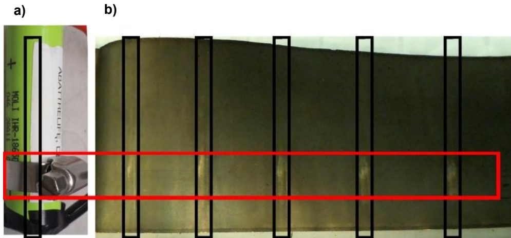
Figure 4.15 Localized plating due to external compression. a) A hose clamp is placed on a cell. b) Plating is visible on the overlap of the current collector imprints and the clamp which are visualized by black and red rectangles respectively.
