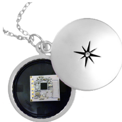
Fig. 6.14 Oncoming prototype of necklace containing Onyx Beacon One inside
