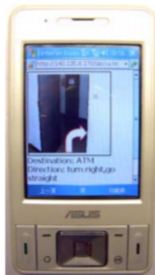
Fig. 2.8 An image with direction is shown on the PDA (Context-Aware Wayfinder system) (Chang et al., 2008)
