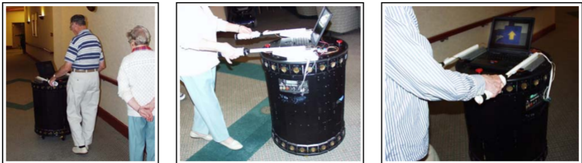
Fig. 2.6 The IMP robotic walker showing a) the robotic walker escorts an elderly person, b) the haptic interface for controlling the walker and c) the walker display with an arrow toward the destination (Morris et al., 2003)
