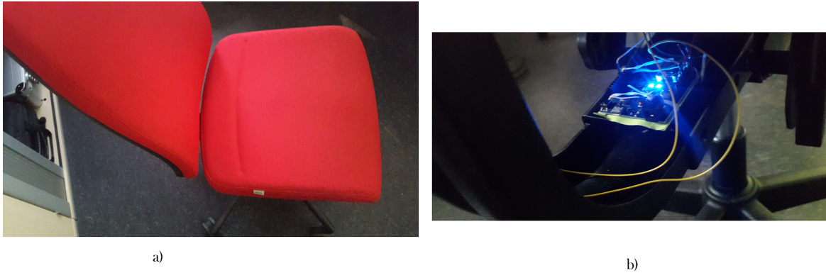
Fig. 6.36 A chair prototype with a pressure sensor (Pololu Force-Sensing Resistor) and an Arduino (WeMos D1-R2). a) The view from above; b) Arduino board under the seat.
