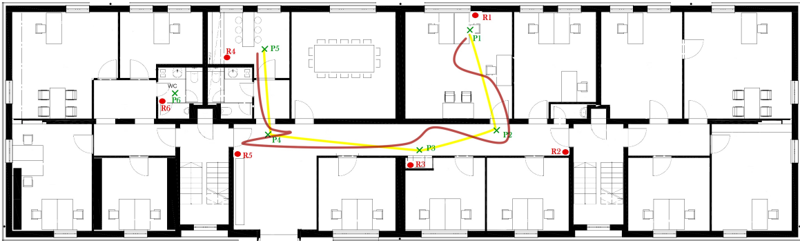
Fig. 6.31 Monitoring system with mobility tracking. Brown line was the route the user moved whereas the yellow line showed the route the system detected and displayed. Readers (R), symbolic locations / reference points (P).
