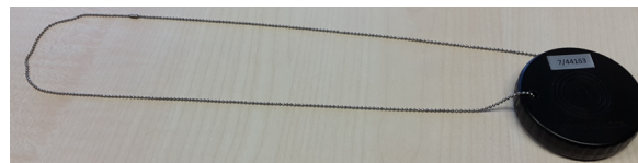
Fig. 6.13 Current prototype of necklace containing Onyx Beacon One inside
