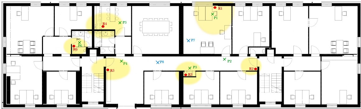
Fig. 6.32 Limiting the detection range of readers to 3-4 meters. Readers (R), symbolic location / reference point (P)
