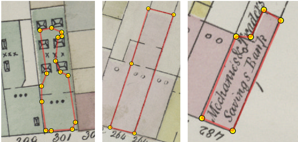
Figure 5.6: The polygon on the left is semantically incorrect because it does not represent a building footprint. The polygon in the middle is also incorrect, because it has one vertex too many. The polygon on the right has inaccurate corner positions, but is semantically correct because it covers the right shape and has exactly one vertex for each corner.
