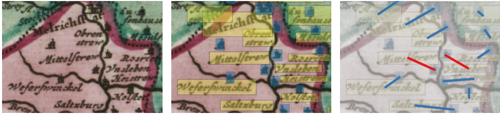
Figure 4.6: Example for an erroneous assignment in experiment CF2: the marker for “Mittelstrew” is matched to the label “Unleben” and vice versa. The map image (left) visually suggests that “Obrenstrew”, “Mittelstrew”, and “Unleben” are each labeled across the river. This assumption can be confirmed by modern map data, since the three villages still exist. Considering the manually created bounding boxes (center), the distances between markers and labels caused by the river become apparent. This, together with the crowdedness of the area, causes the algorithm to fail: it assigns labels vertically along the river rather than across it (right). Also note the unlabeled marker above the “Mittelstrew” label.
