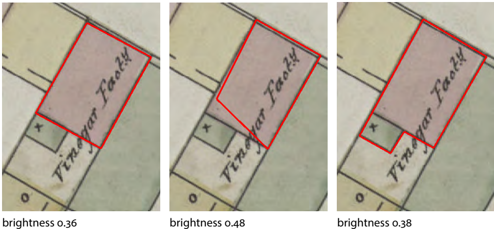
Figure 5.11: The polygon on the left has low average brightness and is semantically correct. The polygon in the center has a worse brightness, but we also consider it to be correct. The polygon on the right has a better brightness, but is semantically incorrect as it marks the union of two footprints.
