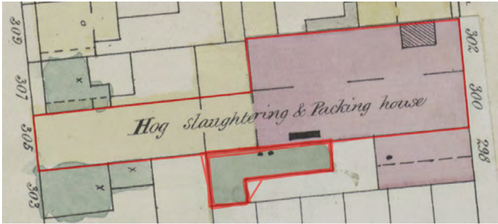
Figure 5.4: The polygons in this group describe two different buildings. There is a single polygon representing the footprint of the Hog slaughtering & Packing house on top, and 50 polygons describing the L-shaped building below (of which one is noticeably imprecise).
