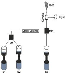
Figure 2-1: Scheme of the Stopped-Flow Setup. S1, S2 and S3 are the syringes, M1 and M2 the mixers and PMT the photomultiplier tube. Figure was modified from Bio-Logic SFM-300/400 user's manual.(Bio-Logic)
