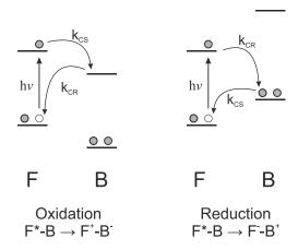
Figure 1-3: Simplified PET-reaction scheme. In the excited state of the fluorophore F\* an electron is either transferred from the higher energy level of the excited state to the electron accepting interactor B (oxidation, left) or from the ground state of B to the ground state vacancy of F\* (reduction, right), resulting in charge separation with the rate kcs. The charge separated system relaxes to the ground state via charge recombination with rate kcs.
