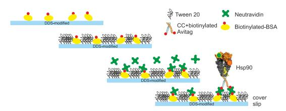
Figure 2-2: Passivation of DDS-coated coverslips. Upper picture shows the first step and lower picture the last step in the protocol. First BSA-biotin is added, followed by Tween 20. Neutravidin is added and finally serves as attachment site for the biotinylated Hsp90-molecule, added in the last step.
