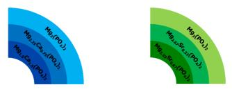
Figure 12: Layer assembly of the  $Ca^{2+}$ - (left) and  $Sr^{2+}$ -substituted (right) struvite tubes in graded samples. View along the tube axis.
