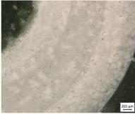
Figure 27: Light microscopy images of  $Sr^{2+}$ -substituted tubes. The outermost layer is a pure struvite cement with an increasing  $Sr^{2+}$  content towards the tube center.
