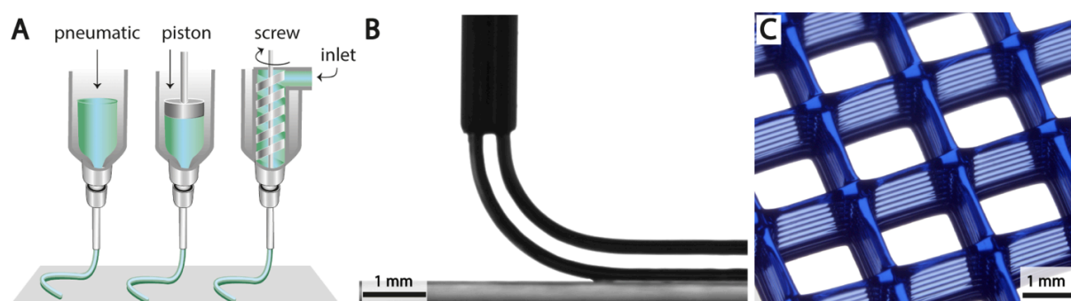
Figure 12: Robotic dispensing A) Schematic drawing of robotic dispensing showing the different mechanisms of ejection. B) Magnified view showing material dispensing from the needle and collection onto a substrate; C) Stereomicroscopic image of a printed Pluronic F127 construct. Reprinted with permission from 39 . Copyright (2016) American Chemical Society.
