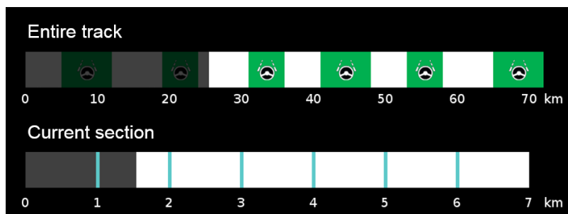
Fig. 4-2: Predictive HMI displayed in the center console. A preview of the entire test track was depicted in the upper area (green sections = automated driving available; white sections = manual driving). A detail view of the current section was shown in the lower area. During the drive, the two bars were filled to highlight the current position. In this example, a third of the whole trip is completed (upper display), the current driving mode is manual (white section) and there are 5.5 km left until a section of highly automated driving (green section) will be reached.
