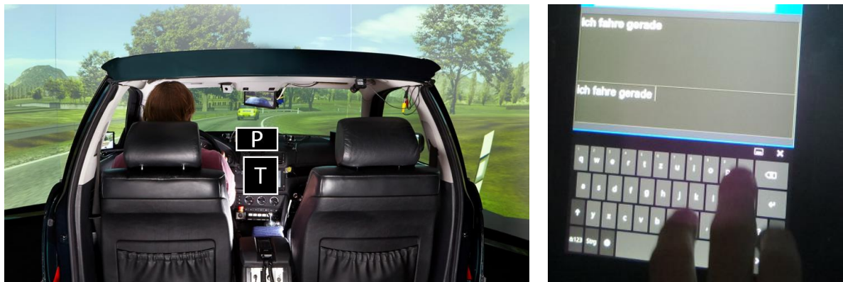
Fig. 4-1: Left: Driving simulator (P = Preview, T = Tablet). Right: Texting task on tablet. Photos: WIVW GmbH.
