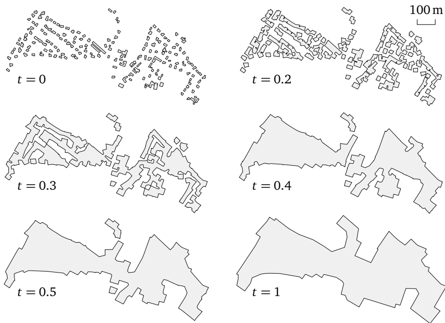
Figure 4.17: Some intermediate-scale results of marked region R_2 in Figure 4.15. When time t = 0.3 , there are some lengthy aggregates.
