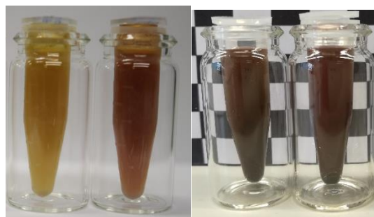
Fig. 70: Diamond conjugates mDND-L1-Ru1c/Ru2b and mDND-L2-Ru1d/Ru2b (from left to right) in aqueous dispersion.
