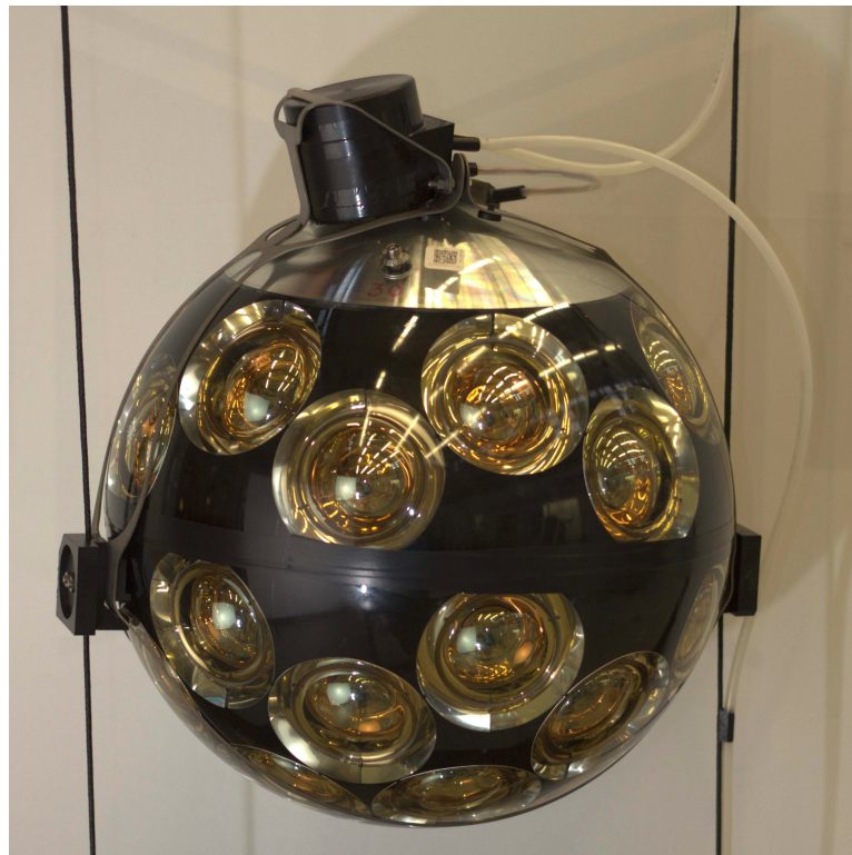
Figure 3.14: Top: Footprint and dimensions of the two sub-detectors ORCA and ARCA of the KM3NeT project. Red dots mark the position of vertical strings. Credit: https://www.km3net.org/km3net-2-0-the-next-phase-arca-and-orca/ Bottom: KM3NeT multi-PMT optical module, containing 31 PMTs as well as all necessary electronics in a 17-inch spherical pressure vessel, mounted between two dyneema ropes. Credit: Adrián-Martínez et al. (2016)
