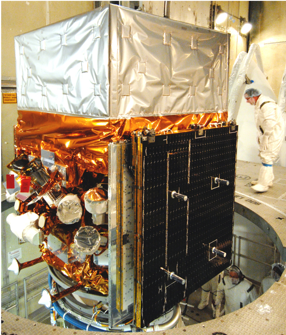
Figure 3.4: Top: Artist illustration of the Fermi Gamma-ray Space Telescope. Bottom: The satellite shortly before launch with the Large Area Telescope (LAT) on the top, the Gamma-ray Burst Monitor (GBM) at the bottom left side and the solar panels folded on the bottom right side of the instrument. Credit: Top: NASA/Sonoma State University, Aurore Simonnet, Bottom: NASA, DOE
