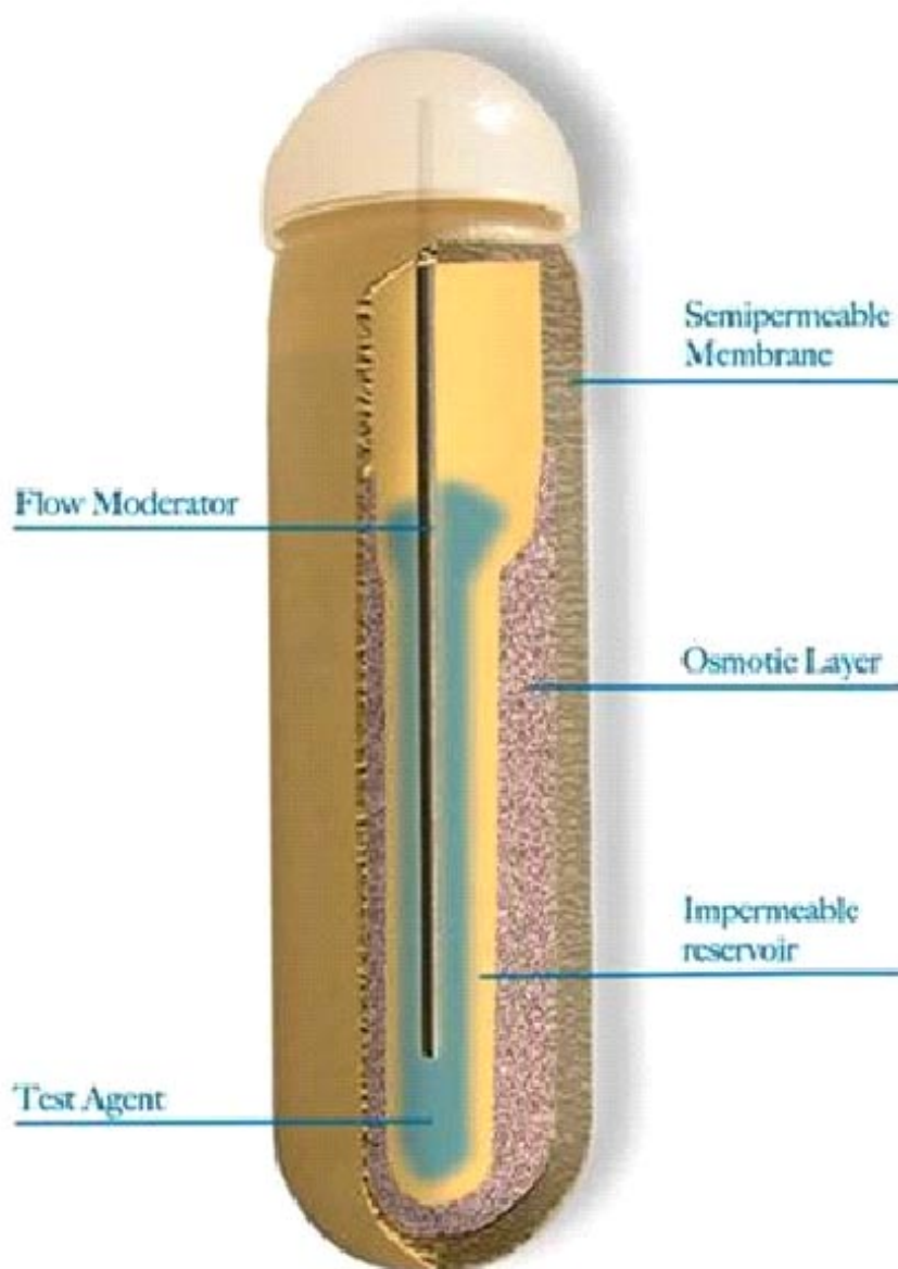
Fig 2.2. ALZET pump. The mini pump have 3 concentric layers: Rate-controlling, semi-permeable membrane; Osmotic layer and Impermeable drug reservoir as indicated. ALZET pumps work by osmotic displacement. Water enters the pump across the outer, semi-permeable membrane due to the presence of a high concentration of sodium chloride in the osmotic chamber. The entry of water causes the osmotic chamber to expand, thereby compressing the flexible reservoir and delivering the drug solution through the delivery portal.
