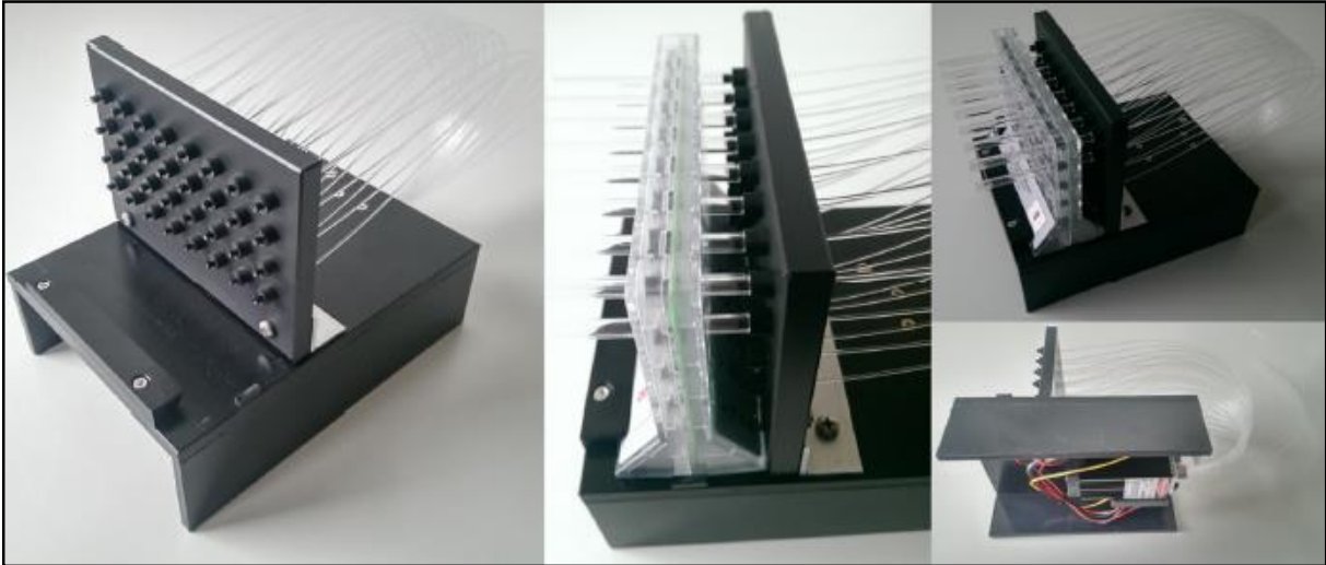
Figure 2.2. Depiction of the used laser application devices; glass fibres extend from the laser directly into the glass tubes, ensuring equal illumination angles; image taken from Dennis Segebarth, Bachelor's thesis [121]
