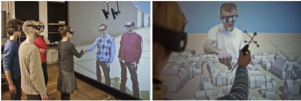
Figure 2.8: An example of a telepresence system from Beck, Kunert, Kulik, and Froehlich [25]. Users are sensed by RGB-depth cameras to reconstruct their appearance and behavior in virtual interactions. Reprinted with permission. Copyright ©2013, IEEE.
