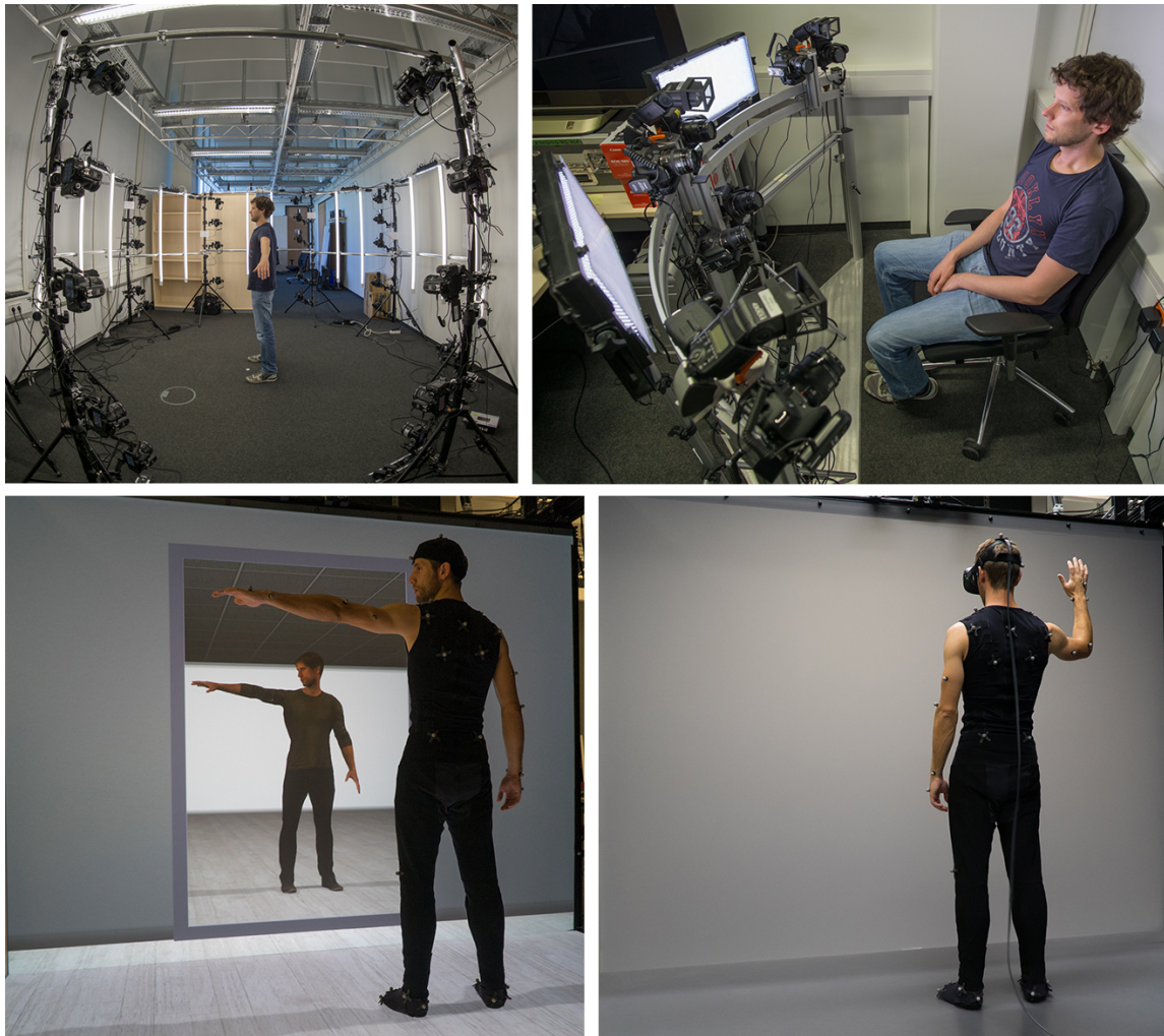
Figure 3.6: Scanning rig and apparatus for the simulation. Left. Separate photogrammetry scans from the face and the body are combined for the creation of the avatar. Right. The user is tracked through body motion tracking (OptiTrack Prime Sense 13W) technology. In the L-shape condition, a stereoscopic L-shaped screen (front, floor) displays passive stereoscopic images. In the HMD condition, the HMD displays the simulation to the user. The two top figures are reprinted from [174] © 2017 Latoschik, Achenbach, Botsch et al.; the two bottom figures are reprinted from [348] © 2018 IEEE.
