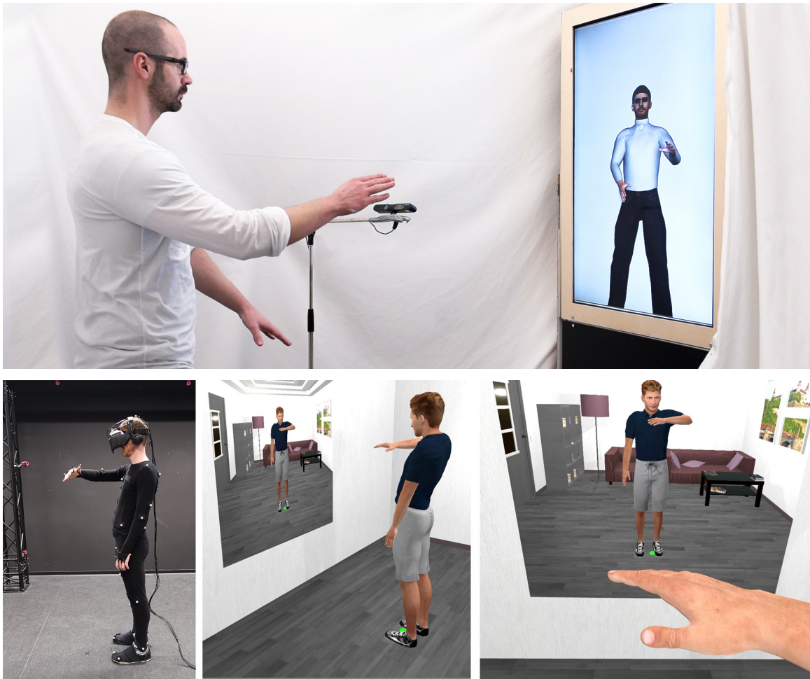
Figure 2.2: Examples of experimental platforms to study virtual embodiment and body ownership illusions. Top: A fake mirror system using a screen in combination with body and facial tracking (adapted from [173]). Bottom: Immersive HMD-based virtual mirror simulation based on passive optical marker tracking, HMD-based gaze tracking, and lower facial expression tracking.
