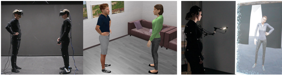
Figure 2.9: Examples of avatar mediated-systems. Left: An immersive system that reproduces behavior to avatars and renders to HMDs. Avatars transmitted can be of different form or gender. Right: A fish tank VR system that reproduces behaviors to avatars and renders to a projection display.
