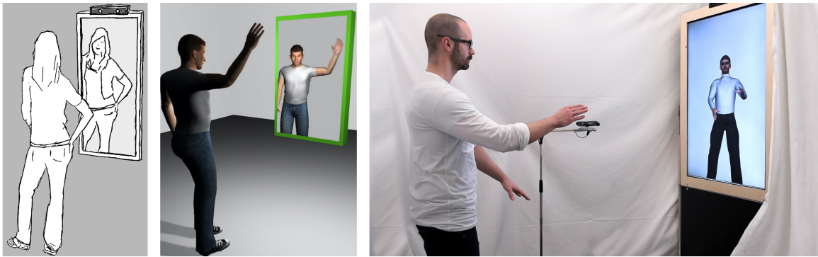
Figure 3.2: The principle of the fake mirror system (adapted from [173], Copyright ©2016 ACM). The user's body movement and facial expression are tracked by sensing technology (Microsoft Kinect V2, PrimeSense Carmine V 1.09a). The simulation retargets these behaviors to avatars. The perspective is rendered according to a fish tank VR principle [353]. A stereoscopic screen displays passive stereoscopic images of the simulation.
