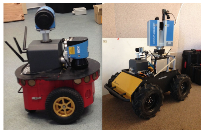
Fig. 1 Intelligent mobile mapping systems. Left: autonomous mobile robot PIONEER 3DX equipped with 3D laser measurement unit. Right: mobile mapping system based on robot Husky equipped additionally with accurate geodetic 3D laser Z+F IMAGER 5010
