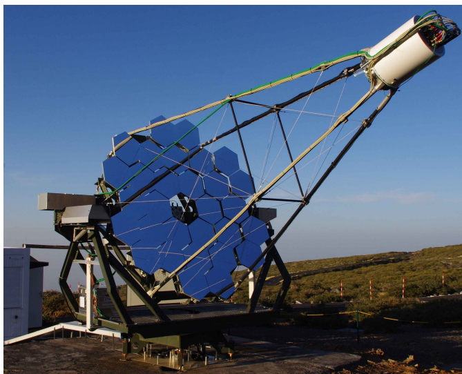
Figure 4.4: The FACT telescope at 2,200 m altitude on La Palma. The 9.5\text{ m}^2 mirror area focuses the Cherenkov light of air shower particles in the camera with G-APD photo sensors. Image from Anderhub et al. (2013a).
