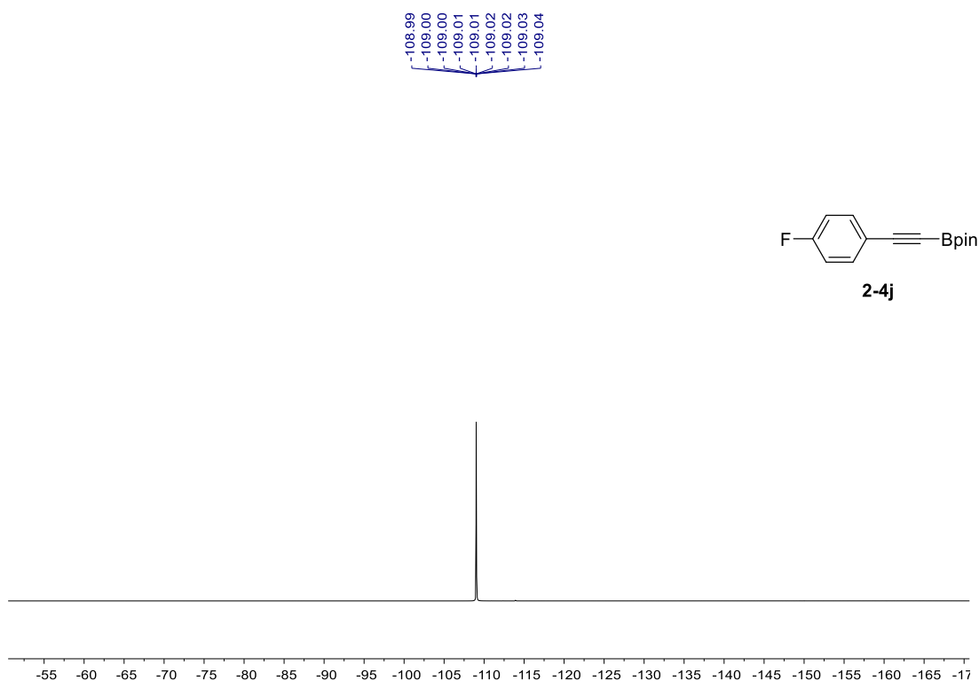
Figure 2-3. ^{19}\text{F} NMR (471 MHz, toluene) spectrum of authentic 2-4j ( \delta -109.0; td, J = 9, 5 Hz).
