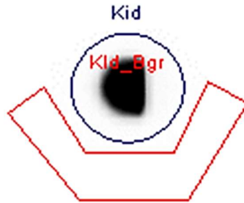
FIGURE 3.5. Post-processing. Exemplary ROI positioning for the kidney phantom (1 y) placed directly on the bed (“Kid”: dark blue) and the background (“Kid_Bgr”: red) [15].
