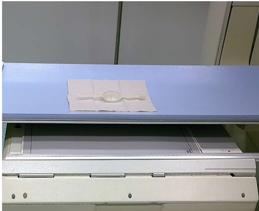
FIGURE 3.4. Phantom experiment. Kidney phantom placed directly on the gamma camera bed (depth position: 0 cm).
