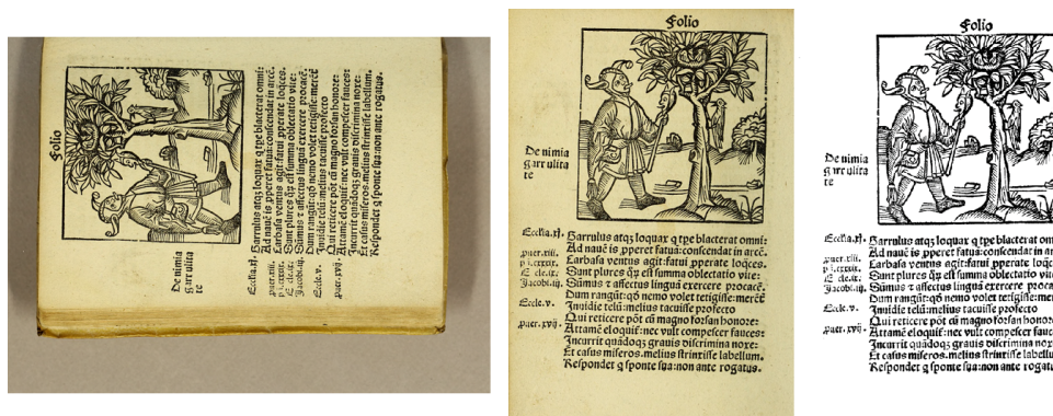
Figure 3. An example input and output of the image preparation and preprocessing steps. The image on the left represents an undesirable input for OCR4all, while the ScanTailor output in the middle is completely sufficient. During the preprocessing step, the skewed color image in the middle is transformed into the deskewed binary image on the right.
