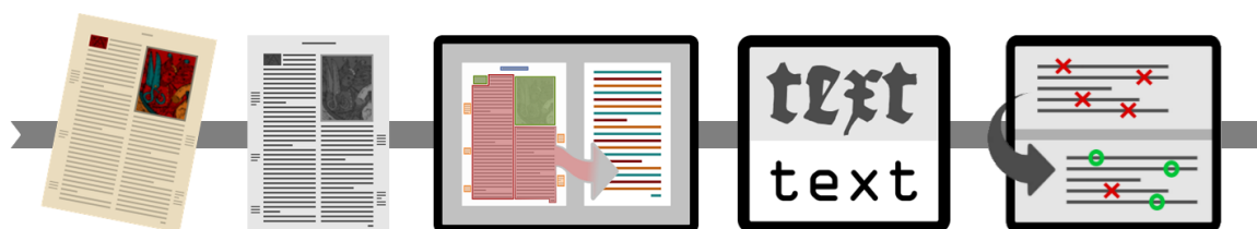
Figure 1. Main steps of a typical OCR workflow. From left to right: original image, preprocessing, segmentation, OCR, postcorrection.
