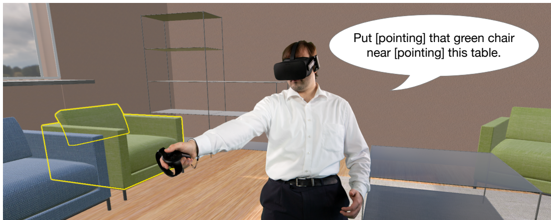
Figure 3. The user is fully immersed into a real-time interactive virtual environment. A multimodal, speech and gesture, interface allows the user to furnish a virtual room.
