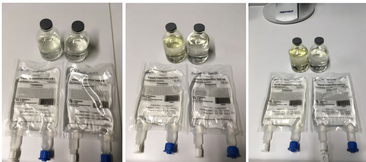
Figure A.5: Image of formulation 1 and 2 (right/left) in glass vials and in plastic bags for injectables. The received pharmaceutical products were redistributed and subjected to the autoclaving procedure (actually a second autoclaving step after the sterilization during manufacturing). From left to right: autoclave time 10 min, 20 min, 30 min, at 121 °C, 2.1 bar. The left samples with formulation 2 showed significantly stronger yellowing than formulation 1, as explained in chapter 3.2.
