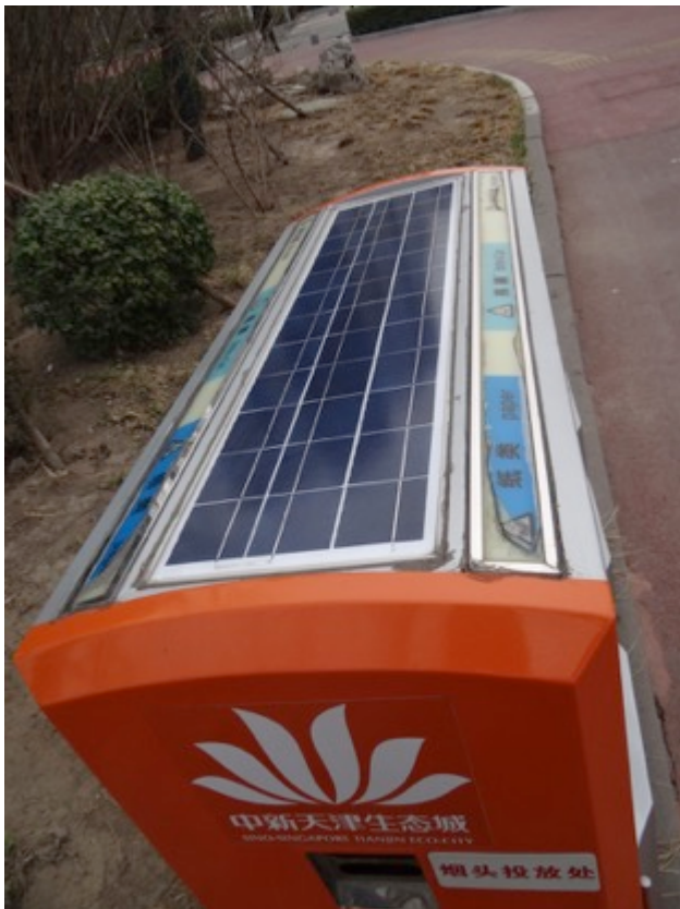
Figure 23: Solar Panels on Garbage Cans in the SSTECC
