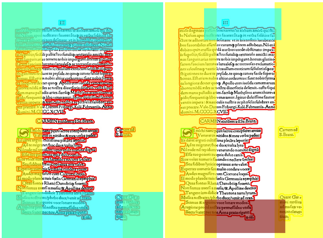
Figure 5.9: Example outcome of the LAREX segmentation when using the default (left) and slightly adjusted (right) parameters. The default setup consists of four regions (image: green, can occur anywhere on the page; paragraph: red, anywhere; marginalia: yellow, left and right 25%; page number: cyan, top and bottom 25%). Naturally, the obtained result is far from optimal and there is still some work to be done. The swash capital was correctly detected as was the page number. However, the marginalia regions got classified as paragraph, as their outer contour was not located entirely within the marginalia regions. Furthermore, there is a signature mark at the very bottom of the page. Lastly, the vertical spacing between text lines is relatively big, leading to the unwanted separation of text blocks. The default setup can be easily adapted by only a few clicks. First, the page number position at the bottom is deleted and the upper one is slightly adjusted, as in this book page numbers always occur at the top center of the page. Furthermore, the marginalia regions have to be expanded towards the middle of the image. The dilation parameters are slightly increased. Finally, another region of the type signature-mark (maroon) is added and located at the bottom center of the page. Adopted from [232].
