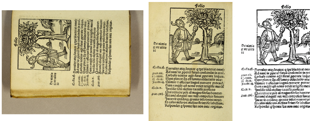
Figure 5.4: An example input and output of the image preparation and preprocessing steps. The image on the left represents an workable but undesirable input for OCR4all while the ScanTailor output in the middle is completely sufficient. During the preprocessing step the skewed color image in the middle is transformed into the deskewed binary image on the right. Adopted from [229].
