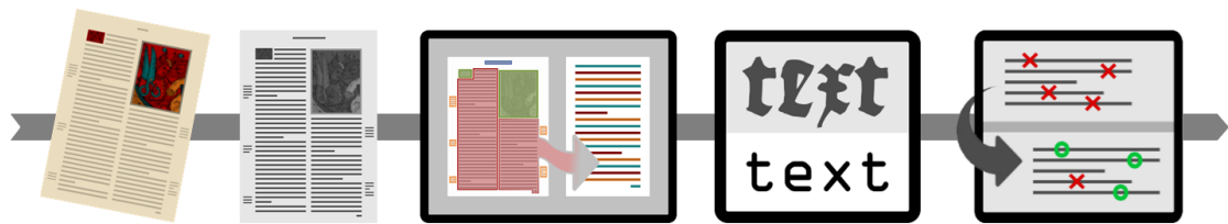
Figure 1.1: Main steps of a typical OCR workflow. From left to right: original image, preprocessing, segmentation, ATR, postcorrection. Adopted from [229].
