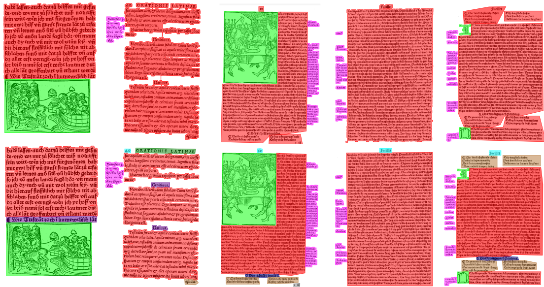
Figure 6.4: Representative example image of three books showing the difference between the basic (top row) and exact (bottom row) segmentation approach. From left to right: P1484, C1541, and N1506 (three images). Adopted from [229].
