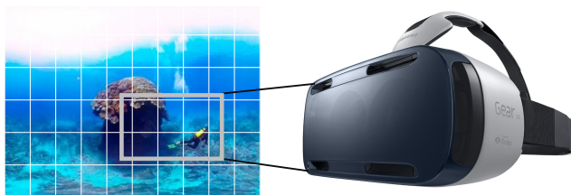
Figure 3.4: Viewport of an HMD on an equirectangularly formatted 360° video. The viewer only sees a subset of all tiles at any point in time.
